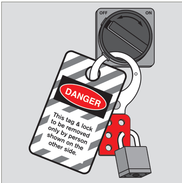
Figure 9 – Example of tagged safety lock-out hasp
