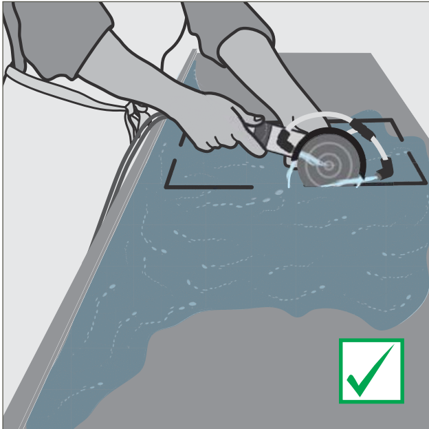
Figure 6(a): Suitable water suppression: grinder being used to cut slab
