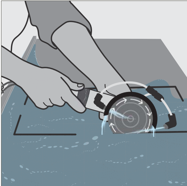
Figure 8: Good spray control – guarding deflects water down towards the slab
