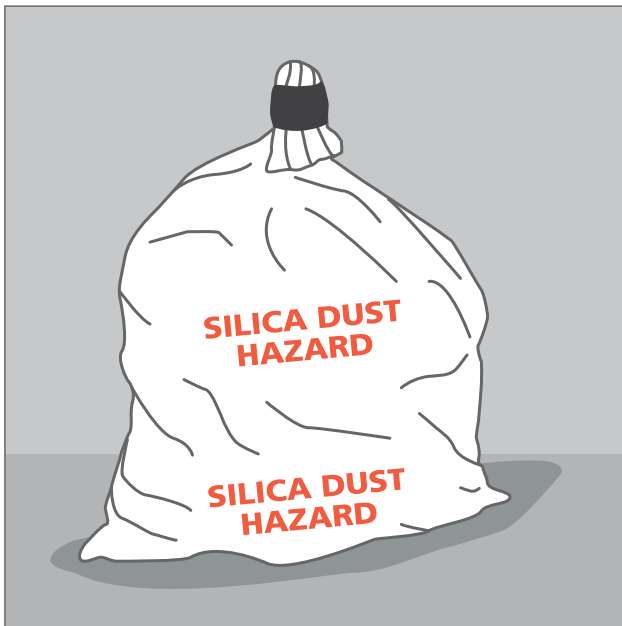
Figure 18: Waste contaminated by silica dust needs to be bagged and labelled
