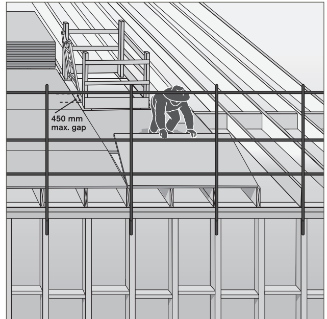
Figure 12 Laying sheet flooring at upper level.
