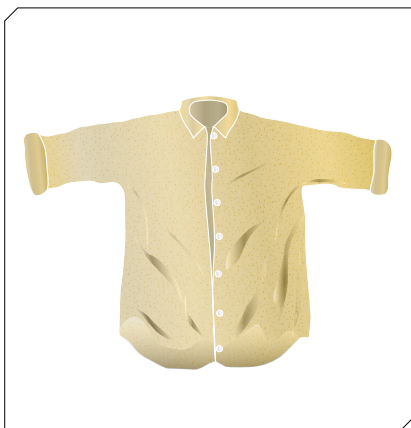
Figure 3: Wool viscose shirt (one example of a flame-resistant fabric) after molten metal pour
