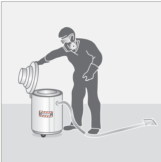
Figure 7: PPE controlling operator exposure and body contamination during short term and infrequent tasks
