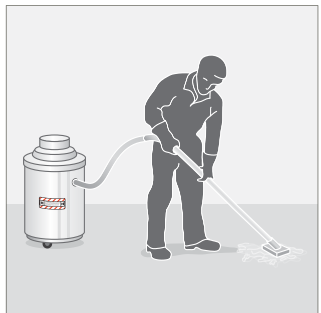
Figure 9(b): After – A hazardous dust class vacuum cleaner
