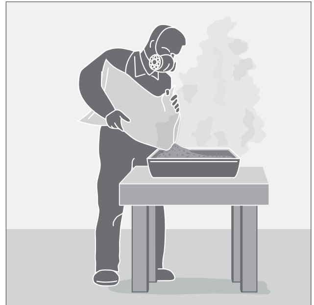
Figure 1(a): Before – dispensing dry lead chemical into a raw material creates airborne dust
