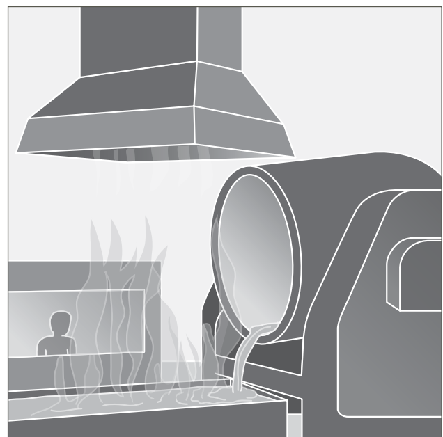
Figure 3(b): After – Isolating the employee from the lead process in a ventilated booth
