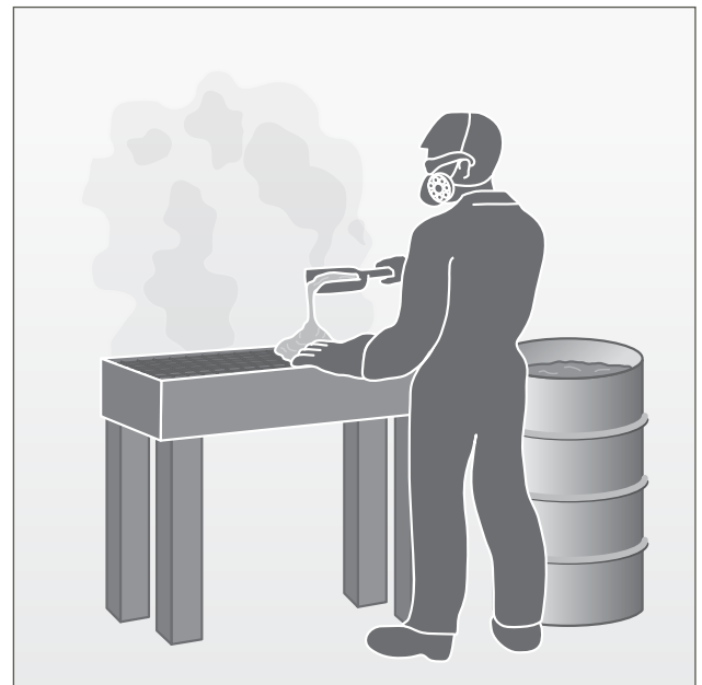
Figure 4(a): Before – Weighing of dry chemical without dust control
