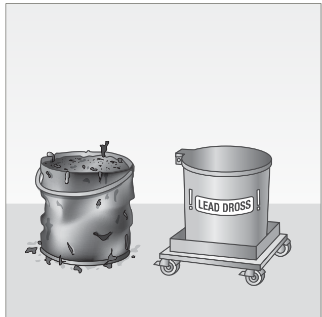
Figure 8: Keeping lead dross in enclosed containers reduces the spread of lead contamination
