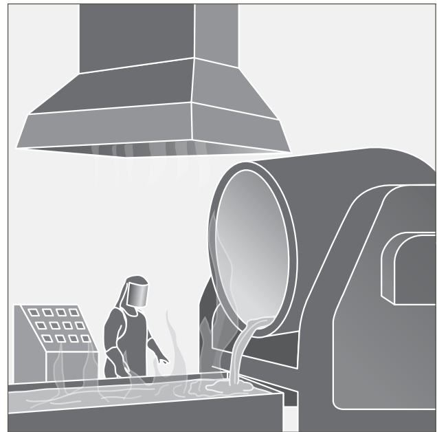
Figure 3(a): Before – Employee working in an area where lead fumes are being produced
