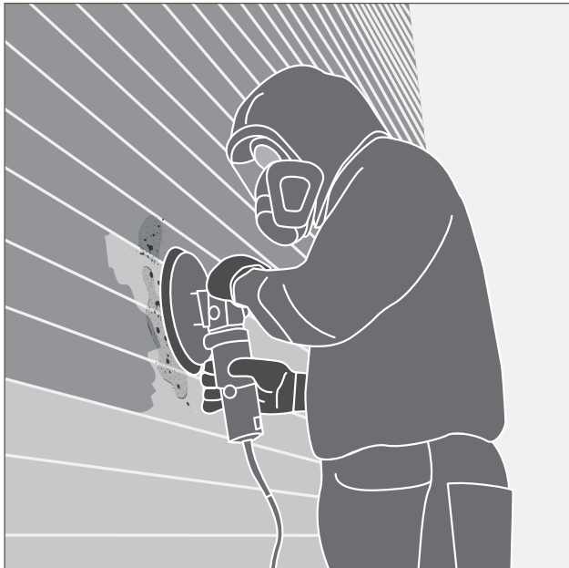
Figure 2(a): Before – using dry powered tools to remove lead-containing paint creates airborne dust
