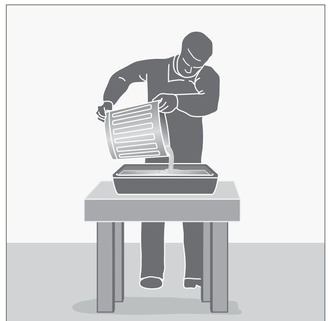
Figure 1(b): After – The use of the lead chemical in a slurry reduces exposure to airborne dust
