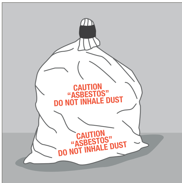
Figure 10: An asbestos waste bag with appropriate warnings.
